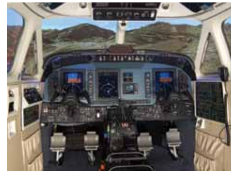
The King Air 350 simulator is equipped with a Collins ProLine 21 avionics panel.
